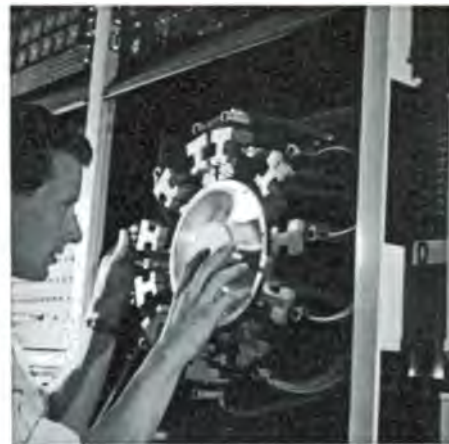
Magnetic drum register-translator: one of the magnetic drums which determine the routes to be taken by calls from London over the network of circuits to all parts of Britain.
