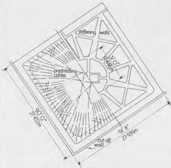
Foundation plan showing stiffening walls and reinforcement ( \frac{1}{4} in = 1ft). Metric equivalents are indicated with dimensions
