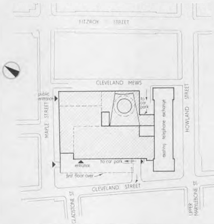
Site plan showing new work adjacent to the existing telephone exchange in Howland Street (1/2" = 1ft)
