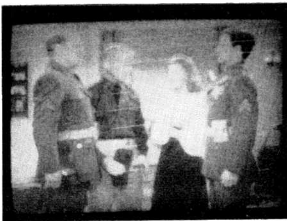
FIG. 1. BRIGHTNESS CONTROL TOO FAR ADVANCED The definition is poor and flyback lines appear on the picture.
