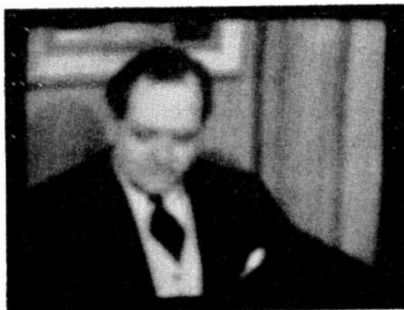
FIG. 2. INCORRECT FOCUSING The line structure is not visible and there is loss of resolution in the picture.
