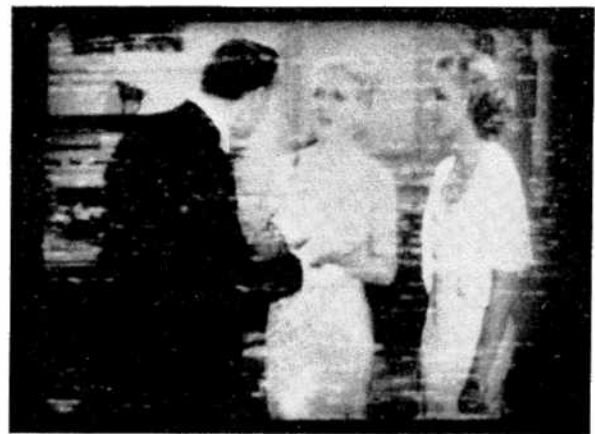
FIG. 23. INTERFERENCE FROM SPARK-TYPE DIATHERMY APPARATUS
