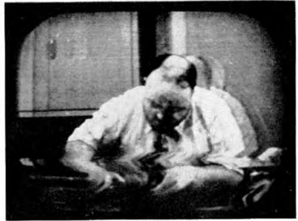
FIG. 31. MULTIPLE IMAGES CAUSED BY MULTI-PATH RECEPTION
