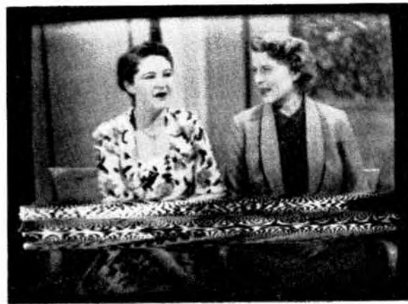
FIG. 27. INTERFERENCE FROM A VACUUM LAMP An oscillating lamp produces a distinctive type of pattern on the picture in very narrow bands.
