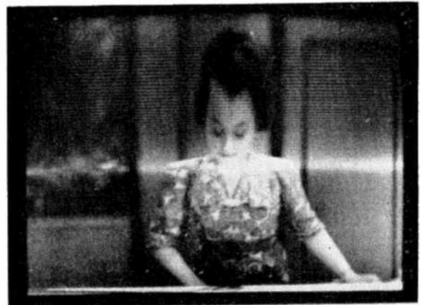
FIG. 8. FRAME LINEARITY CONTROL INCORRECTLY ADJUSTED
