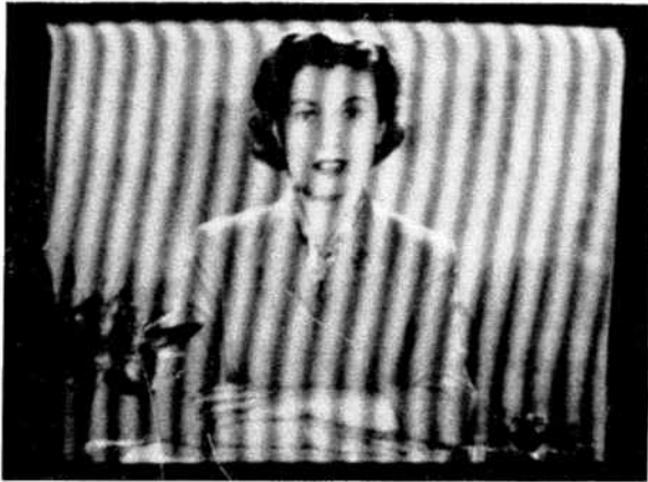
FIG. 33. RADIO TRANSMITTER INTERFERENCE
