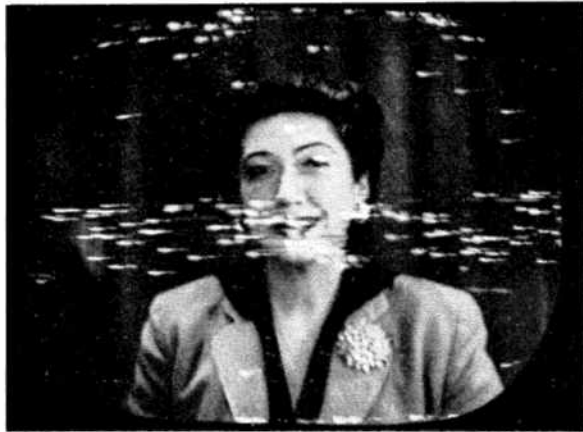
FIG. 20. INTERFERENCE FROM HIGH-VOLTAGE OVER- HEAD POWER LINES
