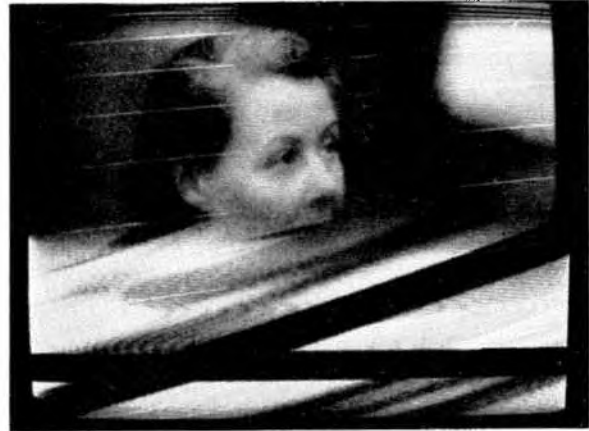
FIG. 26. INTERFERENCE FROM VALVE-TYPE DIATHERMY APPARATUS
