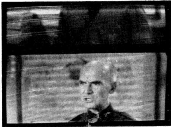
FIG. 6. FRAME (OR VERTICAL) HOLD CONTROL INCORRECTLY ADJUSTED
