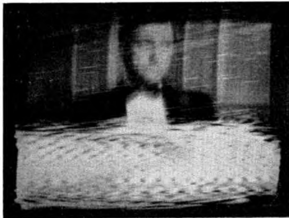
FIG. 25. INTERFERENCE FROM VALVE-TYPE DIATHERMY APPARATUS
