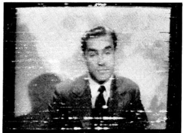
FIG. 16. INTERFERENCE FROM A SEWING-MACHINE MOTOR
