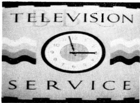
FIG. 9. LINE AMPLITUDE (OR PICTURE WIDTH) CONTROL INCORRECTLY ADJUSTED
