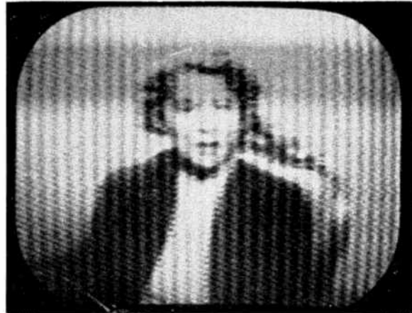
FIG. 35. RADIO TRANSMITTER INTERFERENCE
