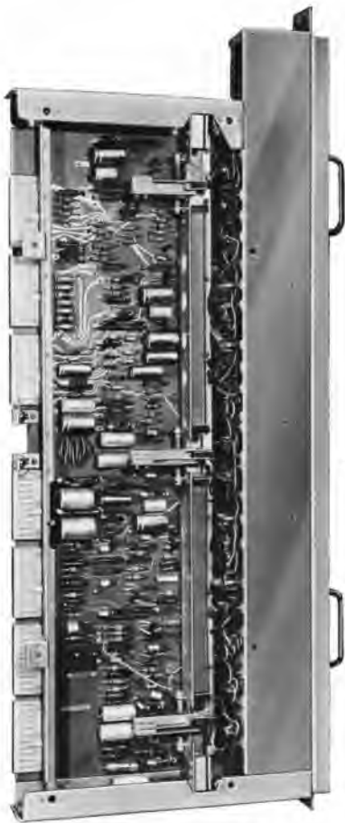
Fig. 1. Typical 100-microsecond delay-line store.
