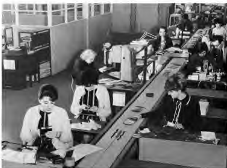
Fig. 2. Track assembly of cards for electronic telephone exchange Mark 2.
