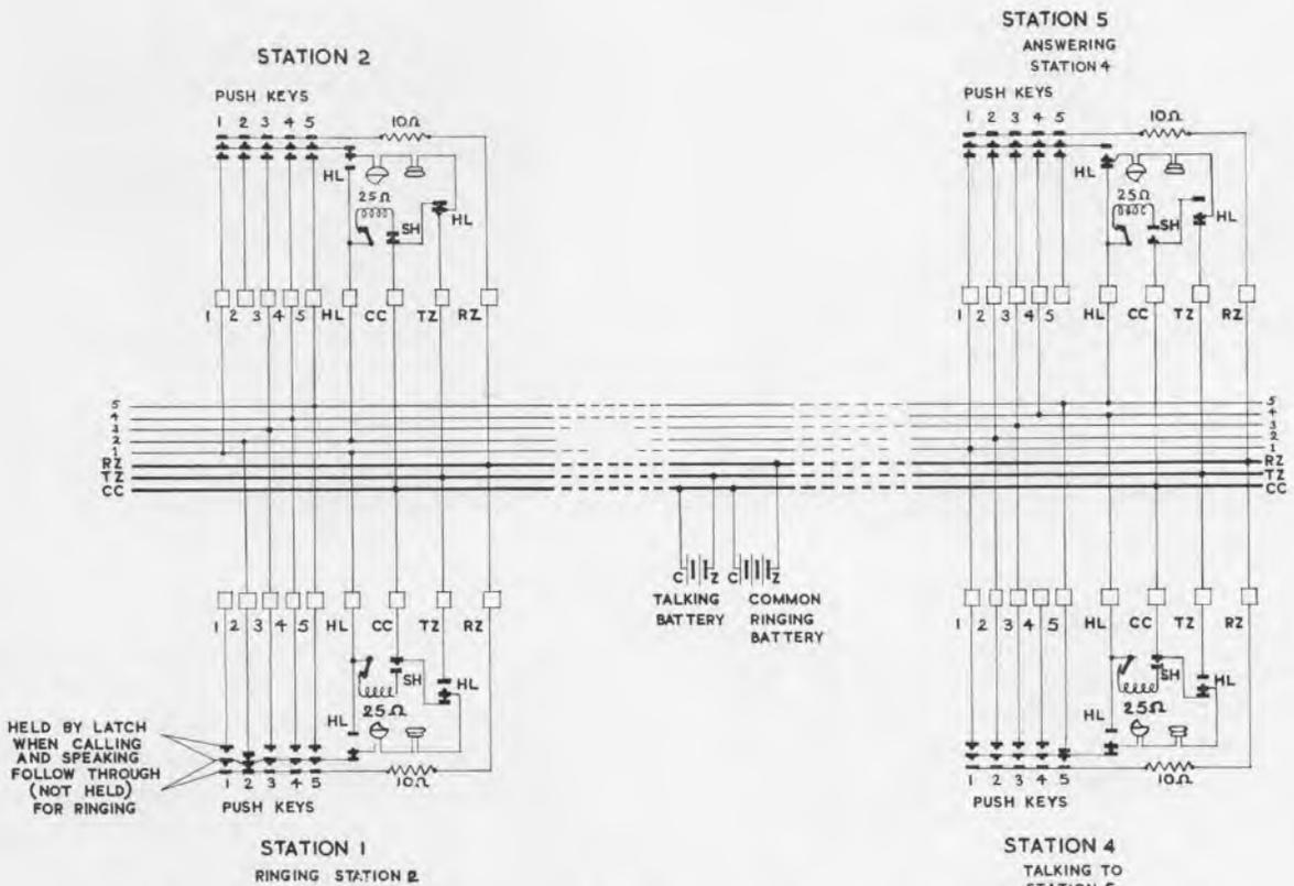
Fig. 4.—Circuit conditions, station 1 ringing station 2, and station 4 talking to station 5.
