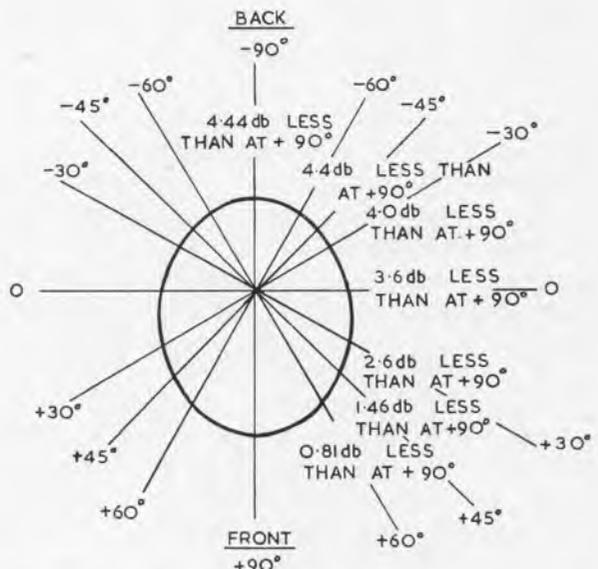
**Fig. 10.—Polar diagram, microphone output, user speaking from constant distance of 8 ft.**
