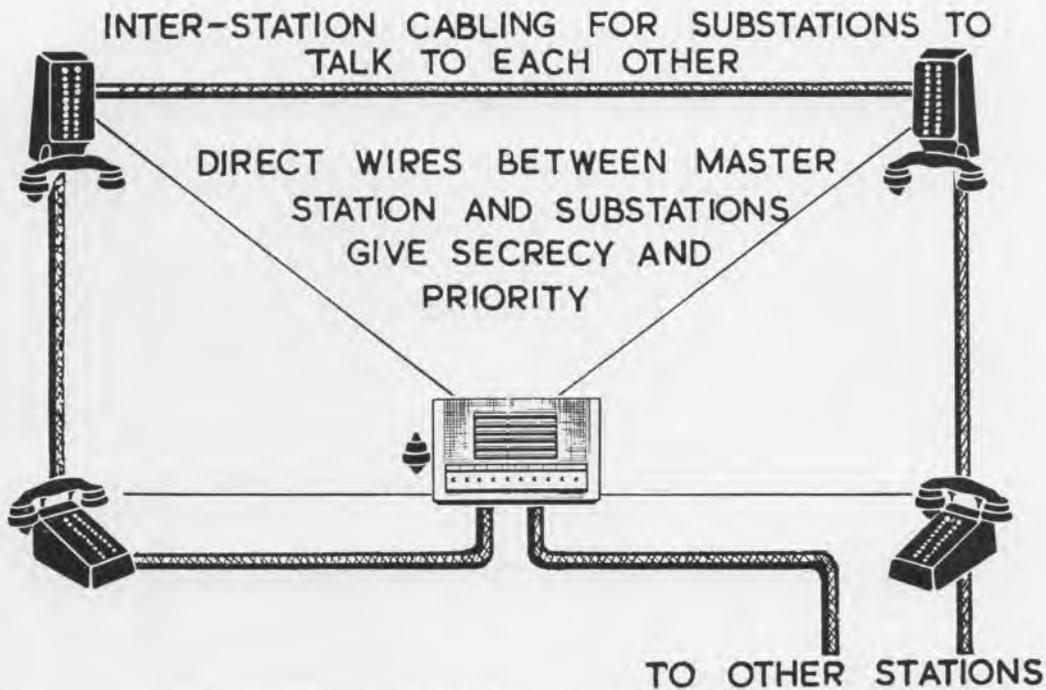
Fig. 11.—Connexions for Loudspeaking Master System.
