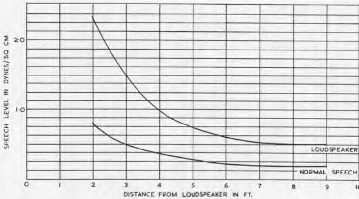
**Fig. 8.—Speech-level/distance curves for loudspeaking telephone compared with normal speech.**
