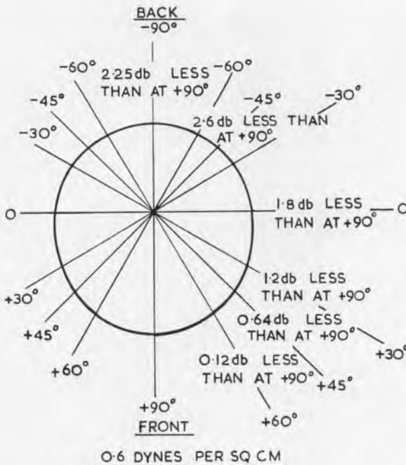
**Fig. 9.—Polar diagram, speech level at constant distance from loudspeaker of 8 ft.**
