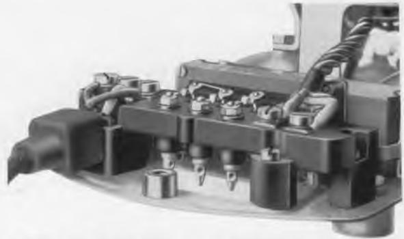
Fig. 6.—Plunger-type terminals of Muraphone, Cat. No. 89A.
