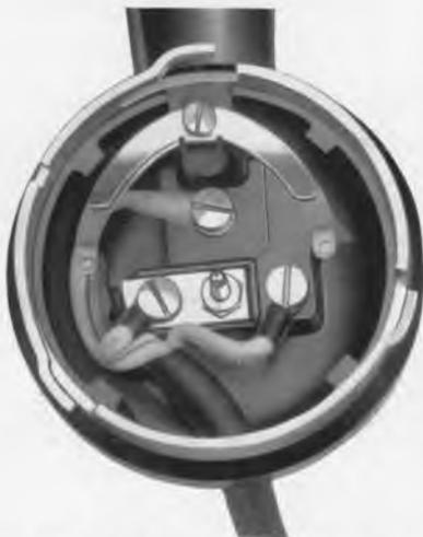
Fig. 5.—Anchorage of handset cord.
