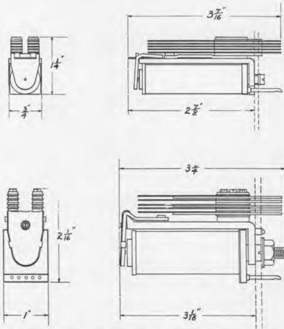
Fig. 2.—Dimensions of the "minor" relay compared with those of the larger type in general use.
