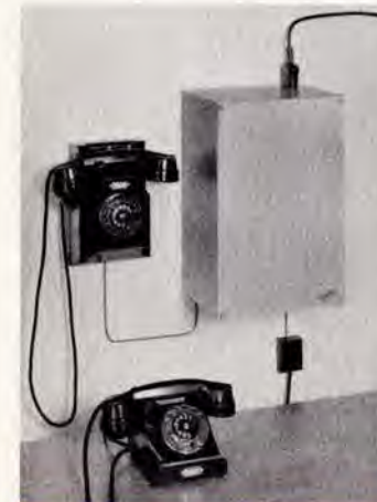
OL 15 serves up to 10 telephones. Dial tone, selective ringing, secret conversation—are features of this system.
