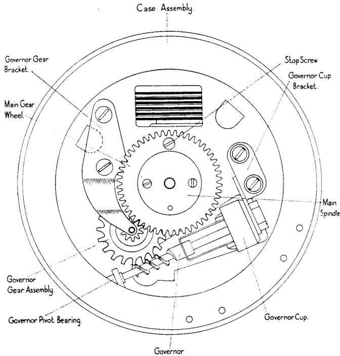
Fig. 3. Front View of the Dial with Finger Plate and Number Ring removed.
