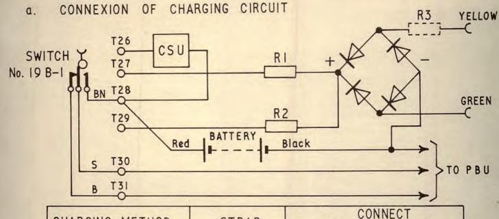
CHARGING METHOD STRAP YELLOW GREEN From line current T26 - T27 T9 T19 T27 - T28 From 10 V power unit PU - ve PU+ ve T28 - T29 From 50V power unit PU -ve PU+ ve
