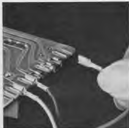
Figure 11 Connection of units to circuit board by push-on leads
