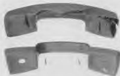
Figure 13. Internal view of two-part handset moulding
