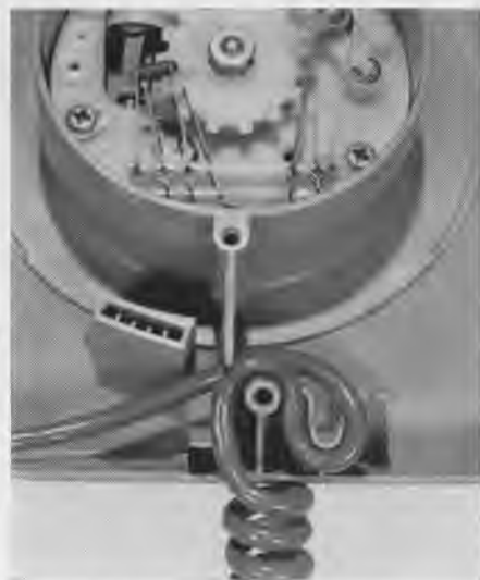
Figure 6. Dial mounting and typical moulded-in grip for positive cord anchorage
