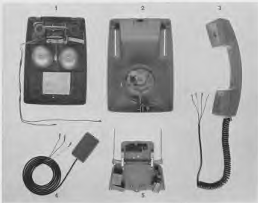
Figure 4. The telephone broken down into its five unit assemblies
