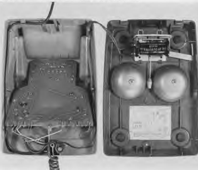
Figure 9. Instrument interior: transmission unit in fixed position.
