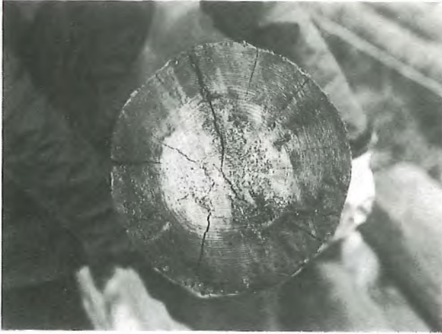
FIG. 4—Cross-section showing shakes penetrating to the heartwood, where decay is well advanced
