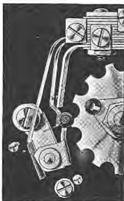
FIG. 12.—TRIGGER MECHANISM—TRIGGER RIDING OVER TOOTH OF PULSE WHEEL AFTER RELEASE OF FINGER PLATE
