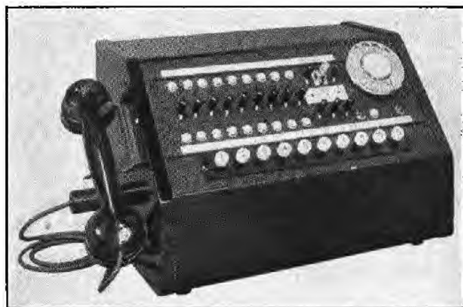
FIG. 3.—THE CORDLESS SWITCHBOARD.
